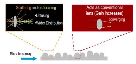
Source: DisplaySearch 2011c Figure 4-12. Mechanism of Micro-lens Films
