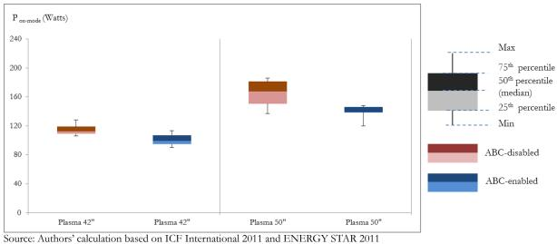
Figure 6-13. On-mode Power of PDP TVs
