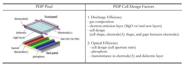
a. Improved Discharge Efficiency (Increased UV Generation Efficiency)
