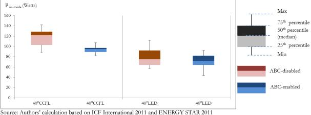
Figure 6-12. On-mode Power of 40-inch LCD TVs
