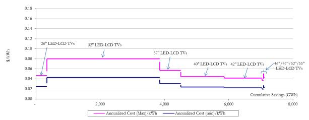
Figure D-2. Cost of Conserved Energy for Dimming Option (2012 LED-LCD TVs)
