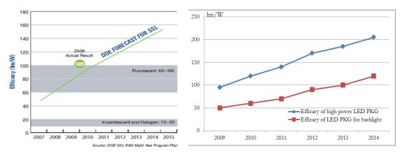
Sources: (left) DOE 2010a; (right) LED manufacturer Figure 4-6. LED Roadmap for Luminous Efficacy (lm/W)
