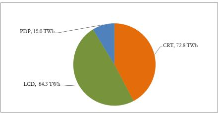
Source: Analysis using the Bottom-Up Energy Analysis System (BUENAS) model Figure ES-3. Global TV Energy Consumption by Display Type in 2012
