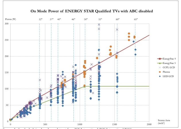
criteria with ABC disabled. In particular, it seems that ABC is important for CCFL-LCD TVs and PDP TVs to meet ENERGY STAR criteria. Figure 6-9 shows on-mode power of ENERGY STAR-qualified TVs with ABC disabled.
