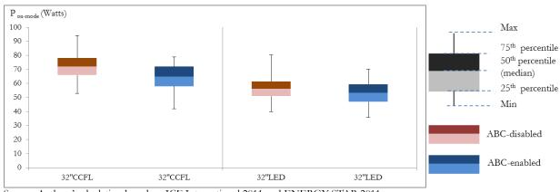
Source: Authors' calculation based on ICF International 2011 and ENERGY STAR 2011 Figure 6-11. On-mode Power of 32-inch LCD TVs with ABC and without ABC
