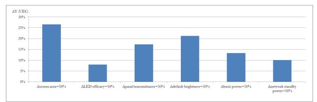
Figure C-1. UEC Sensitivity to Technical Factors (32" LED-LCD TV, P<sub>network standby</sub>=4 W)
