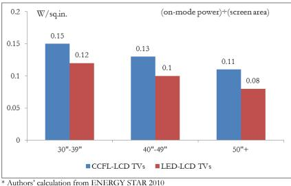
Figure 4-1. Average Watts per Square Inch of LCD TVs by Backlight Type
