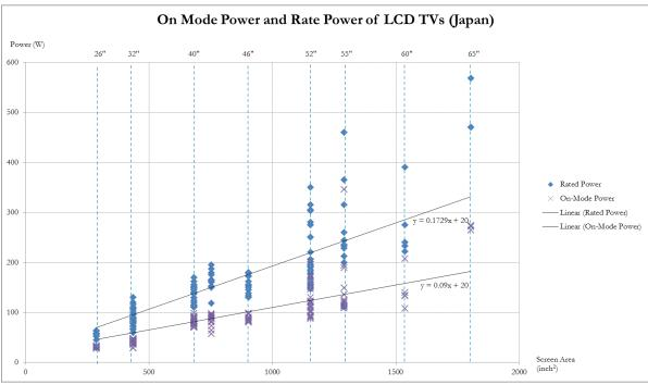
Figure 6-2. On-Mode Power and Rated Power of LCD TVs (Japan)
