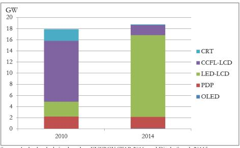
Source: Author's calculation based on ENERGY STAR 2011a and DisplaySearch 2011f Figure 2-15. Total On-Mode Power by TV Market Forecast without Efficiency Improvement
