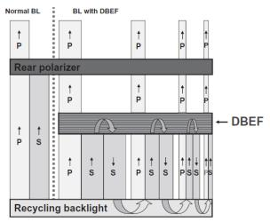
Source: Hanzawa 2009 Figure 4-11. Utilization of Light With and Without a DBEF
