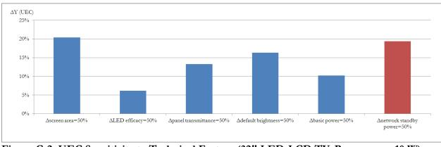
Figure C-2. UEC Sensitivity to Technical Factors (32" LED-LCD TV, P<sub>network standby</sub>=10 W)
