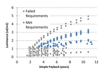
A Canadian municipality used the tool to identify fixtures that met lighting performance criteria – these were up to 74% more efficient than the existing fixture.
